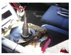
opened the console compartment and guided the two levers for trunk and gas through the opening as I slid the console forward and then over the shift stick and off altogether. The next step was to unscrew the old boot frame and remove the old boot. Or in my case, it was only a year old. I'll find a car to put it on.
